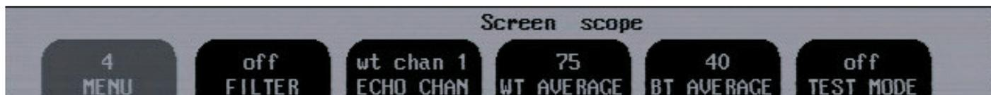
Button 3 is made “active” by pressing the “Hidden button” for 5 seconds, inside the display unit. Press two times untill a “pip” is heard.
